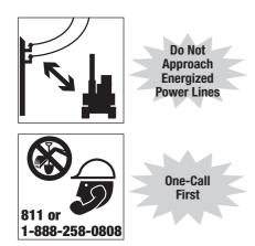
WARNING! Avoid possible injury from contact with buried utilities. Always contact the local One-Call center and any utility companies that do not subscribe to One-Call before digging. Failure to locate existing utilities could result in death or serious injury. (See page 7, One-Call First.)
